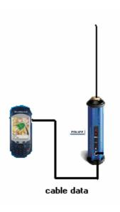
The external battery is not needed as the PDL rover has an internal battery. So the only connection is between the PDL and the ProMark3 using same Pac Crest cable as for the base. (Pac Crest p/n: A02559)
